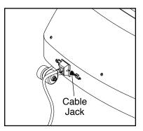
A satellite receiver, VCR, or DVD player can also be connected to the treadmill. Connect a CATV cable from the coaxial output on your equipment (usually labeled TV OUT or RF OUT) to the cable jack on the front of the treadmill.
