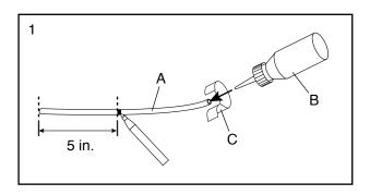
Insert the end of the tubing (A) under the center of the Walking Belt (166). Next, squeeze the silicone bottle (B) while pulling the tubing out from under the Walking Belt until you see the mark on the tubing. Then, remove the tubing from beneath the Walking Belt. Repeat this step on the other side of the Walking Belt.
