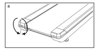
b. If the walking belt slips when walked on, first remove the key and UNPLUG THE POWER CORD. Using the hex key, turn both idler roller screws clockwise, 1/4 of a turn. To properly tighten the treadmill, see step 6 on page 27. Be careful to keep the walking belt centered. Then, plug in the power cord, insert the key, and carefully walk on the treadmill for a few minutes. Repeat until the walking belt is properly tightened.
