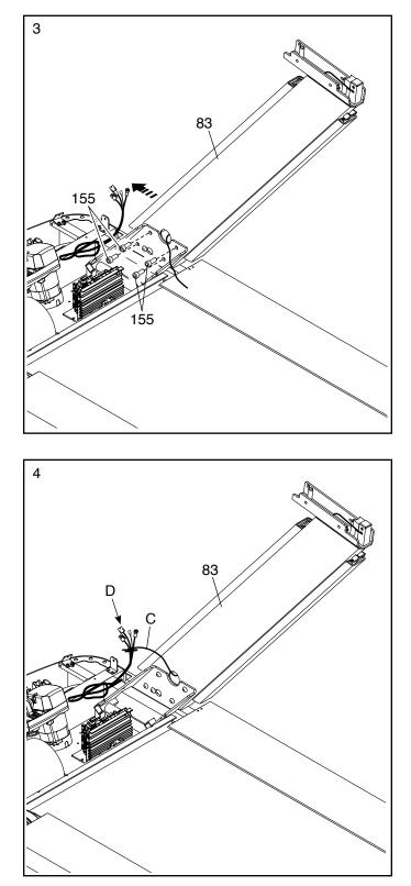
5. With the help of a second person, hold the handrail assembly (E) near the Left and Right Uprights (82, 83). Insert the wires (D) from the Right Upright up through the indicated hole in the handrail assembly.
