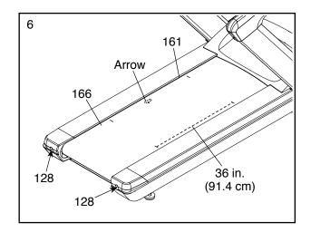
Move the Walking Belt (166), if necessary, until the seam across the Walking Belt is underneath the Walking Platform (161).
