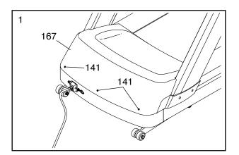
2. Using a handheld vacuum, clean the area under the Motor Hood (not shown). **Be careful to avoid touching any components.** Next, check the Drive Belt (160) for wear and cracks. If the Drive Belt needs to be replaced, see the back cover of this manual.
