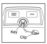
the console, causing the walking belt to slow to a stop. Test the clip by carefully taking a few steps backward; if the key is not pulled from the console, adjust the position of the clip.
