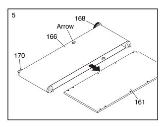
If you are replacing the Walking Platform (161), slide out the old Walking Platform and slide in the new Walking Platform.
