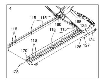
Next, remove the Drive Belt (160) from the Drive Roller (168). Then, remove the two M10 x 110mm Screws (128) from each side of the Idler Roller (170) (only one side is shown). 5. Remove the Idler Roller (170), Drive Roller (168), Walking Platform (161), and Walking Belt (166).
